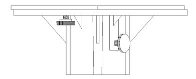
**4. Mounting the equipment on the tripod:** Spread the tripod's legs and ensure that the tripod is stable. Lift the equipment onto the top of the tripod. Tighten the thumbscrew on the side until just snug. Do not over-tighten.
